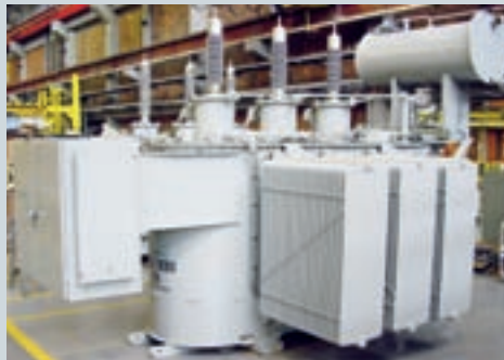
15/20 MVA LDT, 46 +/- 8 x 1.875 % / 6.3 kV, OLTC, for Ecuador
